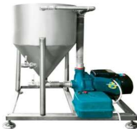
Fig. 2: MFP-200 equipment for the preparation of WMS
