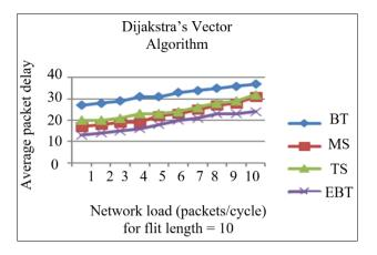
Fig. 15: Average packet delay vs. network load for flit length = 10 in distance vector algorithm
