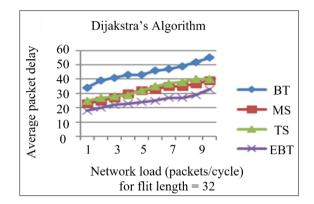
**Fig. 12:** Latency vs. network load for flit length = 32 in Dijkstra's algorithm
