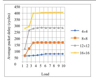
Fig. 20: Average packet delay with an increase in network size (packet size = 32 flits)
