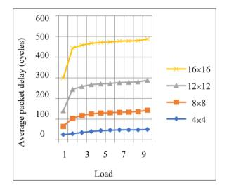
Fig. 19: Average packet delay with an increase in network size (packet size = 10 flits)
