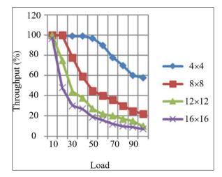
**Fig. 17:** Throughput with an increase in network size (packet size = 32 flits)
