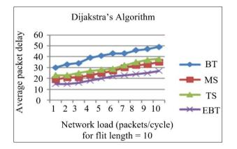
**Fig. 11:** Latency vs. network load for flit length = 10 in Dijkstra's algorithm
