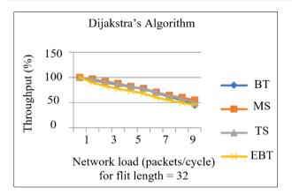
**Fig. 10:** Throughput vs network load for flit length = 32 in Dijkstra's algorithm
