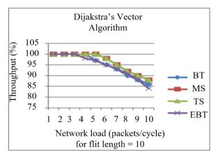
**Fig. 13:** Throughput vs. network load for flit length = 10 in distance vector algorithm
