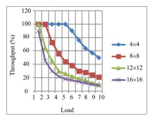
**Fig. 18:** Throughput with an increase in network size (packet size = 10 flits)
