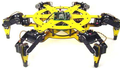
Fig. 1: Body of hexapod robot
