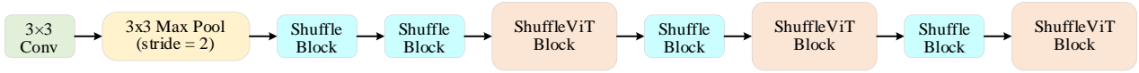
Fig. 11: Structure diagram of multi-head attention mechanism backbone network based on channel rearrangement
